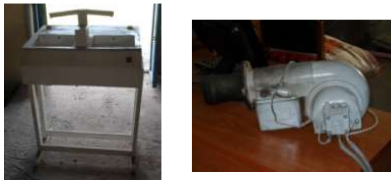
Fig. 1: The automatic hand washing and drying machine with the detached centrifugal chamber beside it
