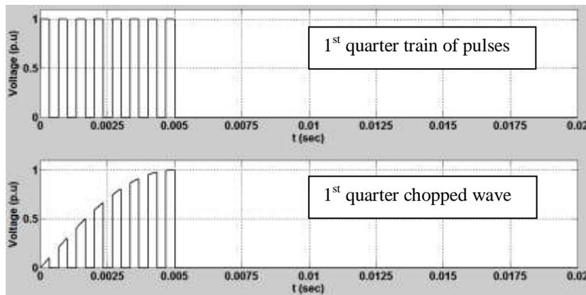
Fig. 1 (a) Developing of first quarter chopped wave
