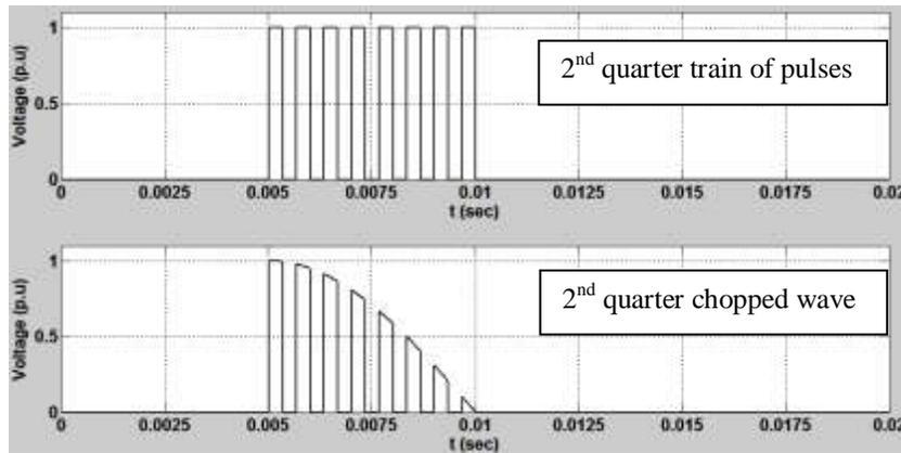
Fig. 1 (b) Developing of second quarter chopped wave
