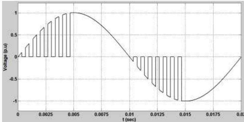
Fig. 12 (a) Output voltage for k = 30, K1 = 0 and k2 = 14, k3 = 0 and k4 = 7
