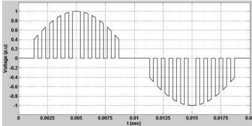
Fig. 7 Output voltage for  $k = 30$ ,  $K1=2$  and  $K2=7$
