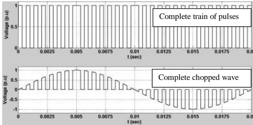
Fig. 2 Development of a full cycle chopped wave
