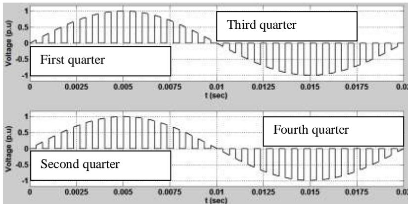
Fig. 6 (b) The four quarters of the output waveform
