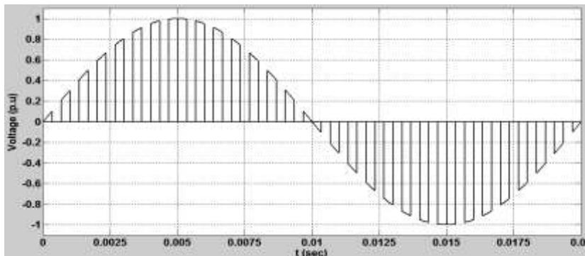
Fig. 3 (b) Combination of the two middle segments in each half cycle
