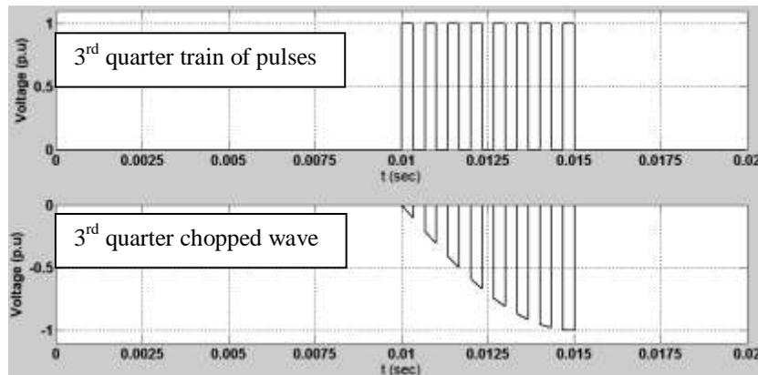
Fig. 1 (c) Developing of third quarter chopped wave
