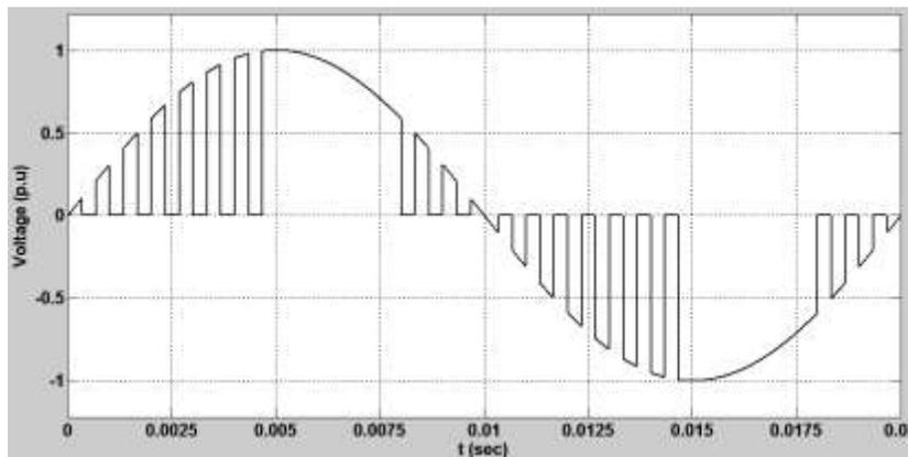
Fig. 12 (d) Output voltage for  $k = 30$ ,  $K1 = 0$  and  $k2 = 11$ ,  $k3 = 0$  and  $k4 = 7$
