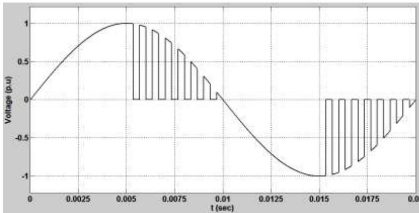
Fig. 12 (c) Output voltage for  $k = 30$ ,  $K1 = 0$  and  $k2 = 7$ ,  $k3 = 0$  and  $k4 = 14$
