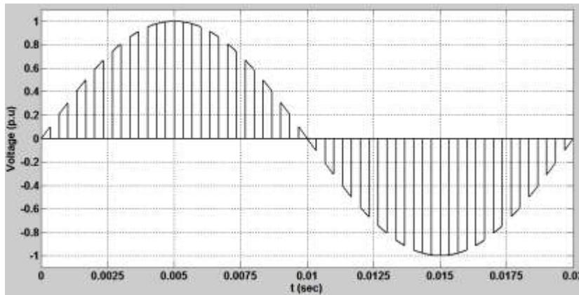
Fig. 4 (c) Combination of the middle segments in each half cycle
