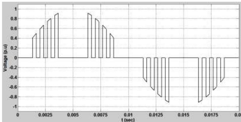
Fig. 10 Output voltage for  $k = 30$ ,  $K1 = 2$  and  $k2 = 5$
