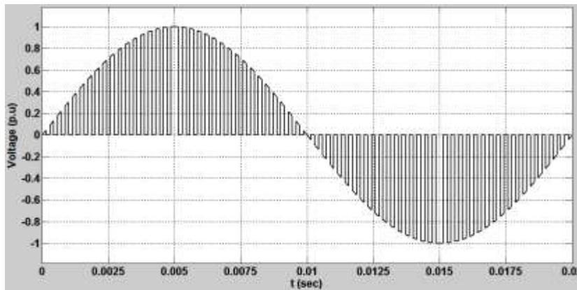
Fig. 11 Output voltage for  $k = 70$ ,  $K1 = 0$  and  $k2 = 17$
