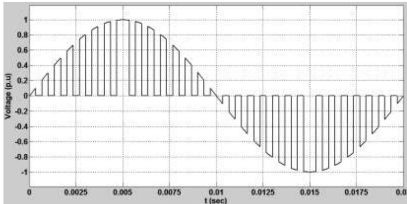
Fig. 3 (a) Output voltage
